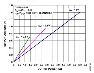
Figure 28. Supply Current vs. Output Power into 4  $\Omega$
