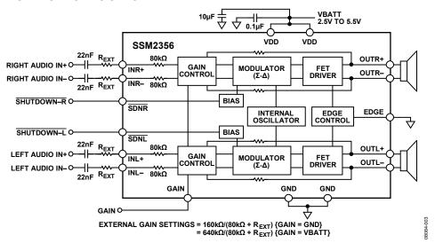
Figure 34. Stereo Differential Input Configuration
