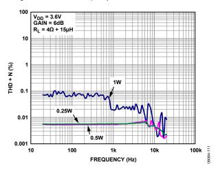
Figure 13. THD + N vs. Frequency,  $V_{DD} = 3.6 \text{ V}$ ,  $R_L = 4 \Omega$ ,  $A_V = 6 \text{ dB}$
