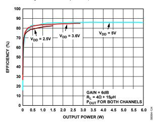
Figure 26. Efficiency vs. Output Power into 4  $\Omega$
