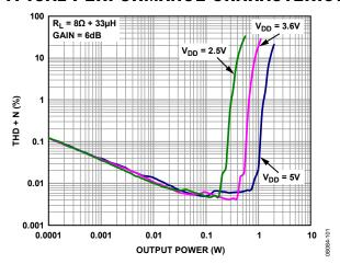
Figure 3. THD + N vs. Output Power into 8  $\Omega$ ,  $A_V = 6 dB$
