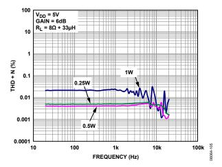
Figure 7. THD + N vs. Frequency,  $V_{DD} = 5 V$ ,  $R_L = 8 \Omega$ ,  $A_V = 6 dB$
