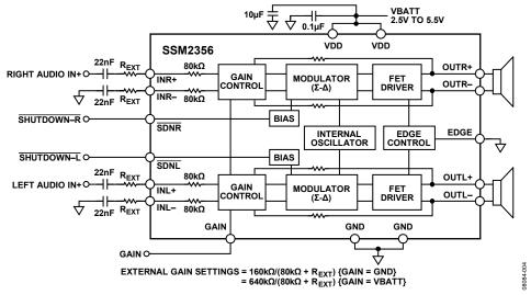
Figure 35. Stereo Single-Ended Input Configuration
