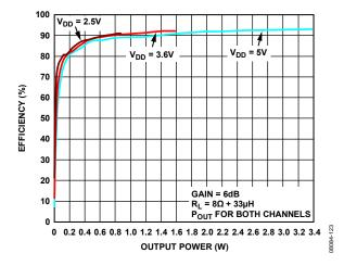
Figure 25. Efficiency vs. Output Power into 8  $\Omega$
