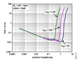
Figure 6. THD + N vs. Output Power into 4  $\Omega$ ,  $A_V = 18 dB$
