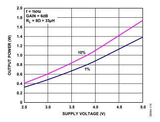
Figure 21. Maximum Output Power vs. Supply Voltage,  $R_L = 8 \Omega$ ,  $A_V = 6 dB$
