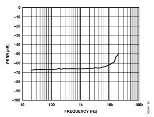
Figure 31. PSRR vs. Frequency
