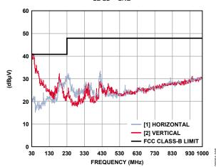
Figure 37. EMI Emissions from SSM2356, 1-Channel, 12 cm Cable,  $EDGE = V_{DD}$
