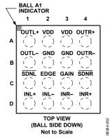
Figure 2. Pin Configuration (Top Side View)
