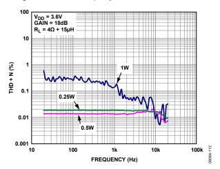
Figure 14. THD + N vs. Frequency,  $V_{DD}$  = 3.6 V,  $R_L$  = 4  $\Omega$ ,  $A_V$  = 18 dB
