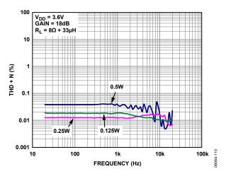
Figure 12. THD + N vs. Frequency,  $V_{DD} = 3.6 \text{ V}$ ,  $R_L = 8 \Omega$ ,  $A_V = 18 \text{ dB}$
