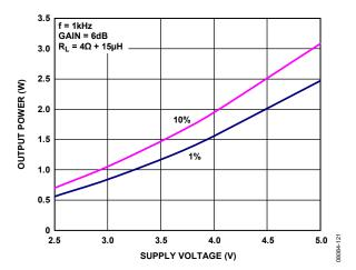
Figure 23. Maximum Output Power vs. Supply Voltage,  $R_L = 4 \Omega$ ,  $A_V = 6 dB$
