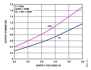
Figure 22. Maximum Output Power vs. Supply Voltage,  $R_L = 8 \Omega$ ,  $A_V = 18 dB$
