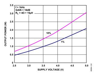
Figure 24. Maximum Output Power vs. Supply Voltage,  $R_L = 4 \Omega$ ,  $A_V = 18 dB$
