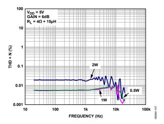
Figure 9. THD + N vs. Frequency,  $V_{DD} = 5 V$ ,  $R_L = 4 \Omega$ ,  $A_V = 6 dB$
