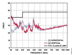
Figure 36. EMI Emissions from SSM2356, 1-Channel, 12 cm Cable, EDGE = GND
